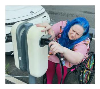
Also consider supporting the weight of the connector while the user is lining it up ready to push into the socket.
